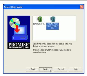
Figure 69. Select the new RAID Level.
